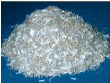
Fig. 1: Free flowing pellets from Cellulose man-made fibers with 4 mm cut length.
