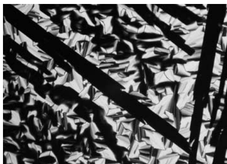
Fig. 2: Optical texture of a binary mixture 1-[4,6]/2 at the transition from the Col h phase to the Cub V2 phase (X1-[4,4] = 0.10) at 176 °C.
