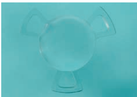
Fig. 3: Blank of an IOL made from the new material with ground-in optics
