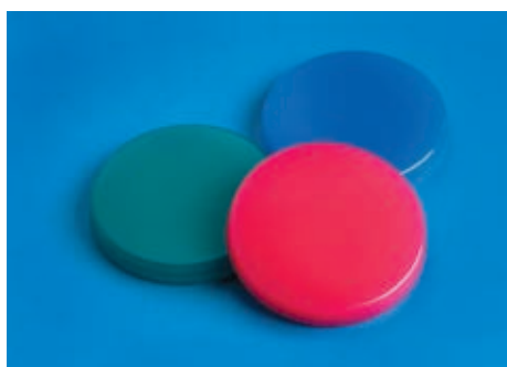
Fig. 2: Samples of thermochromic thermosetting polymers possessing switching temperatures of 60°C.
