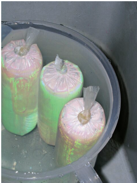
Fig. 1: Monodisperse polymer latex batches: Colors resulting from structure formation after latex cleaning in dialysis tubes.
