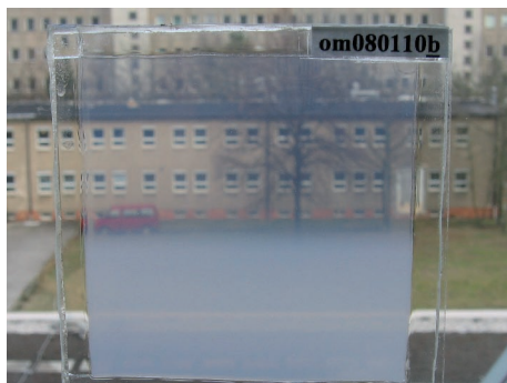
Fig. 3: Example of a laminated glazing with thermotropic properties (underpart heated to 50 °C).
