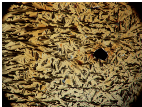
Fig. 2: Optical texture for the rectangular columnar mesophase of equimolar mixed systems of the complementary components.
