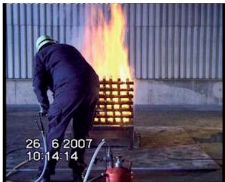
Fig. 2: Attempt to extinguish a fire of a wood frame.
