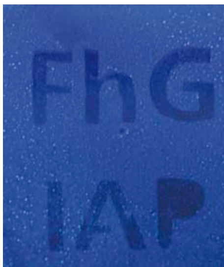
Fig. 3: Cross-linked film emitting blue polarized light under UV illumination: polarizer perpendicular to rubbing direction.
