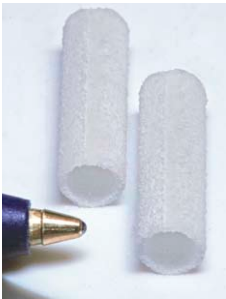
Fig. 3: Prototypes of bioresorbable stents (polymer: polylactide, process: selective laser melting).
