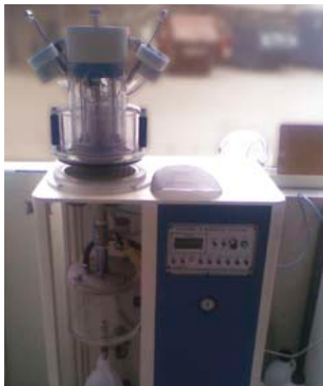
Fig. 2: Paper sheet forming using the »drainage & retention« analyzer.
