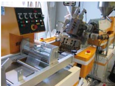
Fig. 3: Manufacturing of polyolefin films by extrusion.
