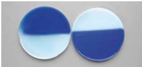
Fig. 1: Conventional (left) and inverse (right) thermochromic switching (above: 20 °C; below: 80 °C) in PE.
