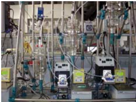
Fig. 2: Lab-scale continuous stirred tank reactor cascade.
