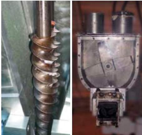
Fig. 1: twin-screw-belt conveyor (ZBFE) and conventional side feeder (ZSFE).
