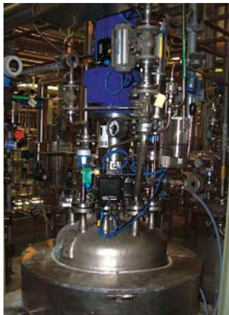
Fig. 1: 670L Pilot plant reactor C2510.
