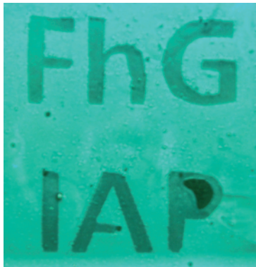
Fig. 2: Thin film of a polarized fluorescent material (original size 4x4 cm) under UV light, viewed through a polarizer perpendicular to the orientation axis of the material.
