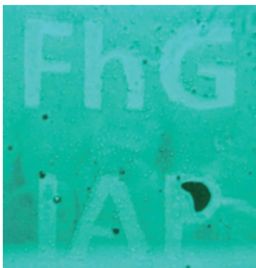
Fig. 3: Thin film of a polarized fluorescent material (original size 4x4 cm) under UV light, viewed through a polarizer parallel to the orientation axis of the material.
