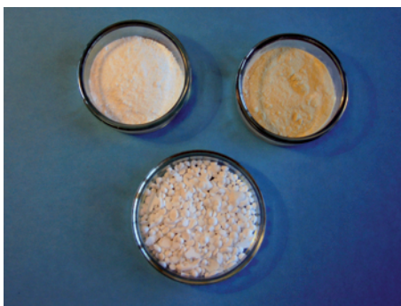
Fig. 1: The three components of a thermochromic leuco dye-developer-solvent system.
