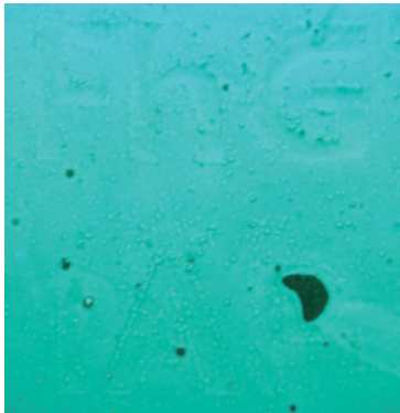
Fig. 1: Thin film of a polarized fluorescent material (original size 4x4 cm) under UV light, viewed without a polarizer.
