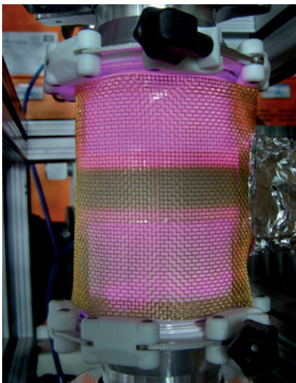
Fig. 2: Plasma reactor for surface oxidation of polyethylene powder.
