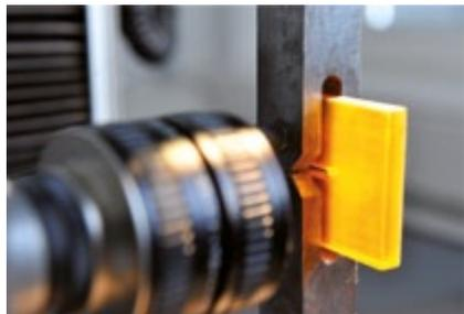
5: Optical Crack Tracing with digital video camera
