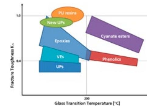
3: Schematic comparison of different classes of unmodified thermosetting resins for fracture toughness and glass transition temperature
