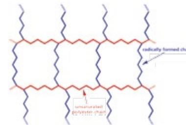
2: Idealized schematic structure of a homogeneous 3-dimensional network
