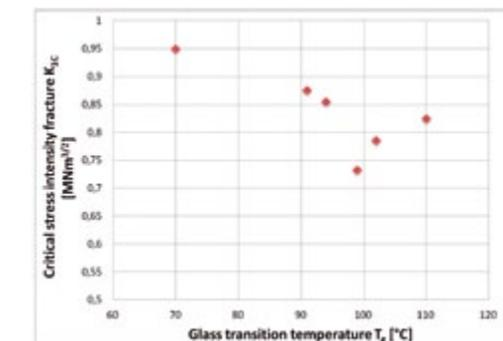
4: Relationship between fracture toughness and glass transition temperature for different new UP formulations
