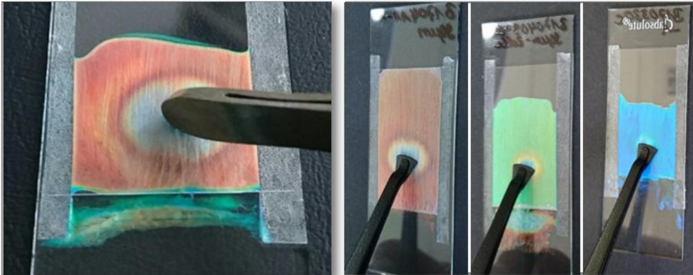
Hypsochromic color change of piezochromic films under mechanical stimulation
