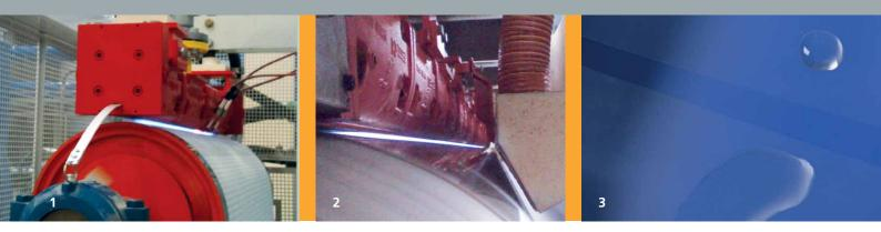
1 Flame treater on a paper extrusion coating line.
