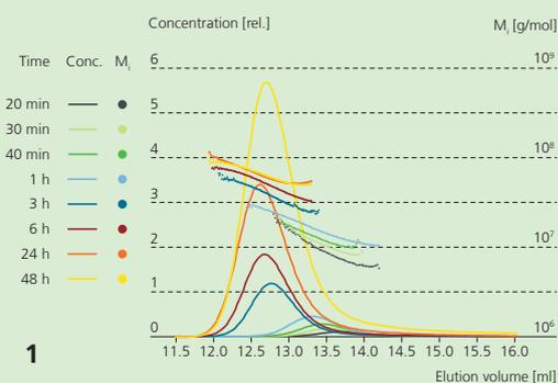
**1** Concentration signal and absolute calibration curves of Inulin depending on the synthesis time.
