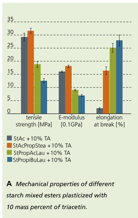
So the elongation at break can be increased by 500 percent in contrast to pure starch acetate (grey) by inserting a propionat and stearat substituent (dark orange) without any loss in tensile strength and stiffness (modulus). By using further internal plasticizer in form of different ester substituents like laurate and i-butyl groups the material gets more and more flexible (green, blue).
