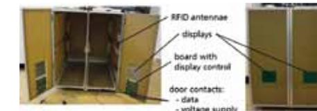
5 Mock-up of a novel galley compartment with bistable displays integrated in the doors
