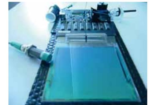
6 Wireless control of a cholesteric reflective bistable display via HF-RFID and with wireless energy transfer via inductive coupling
