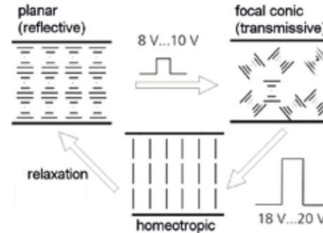
2 Operation principle of bistable cholesteric reflective displays
