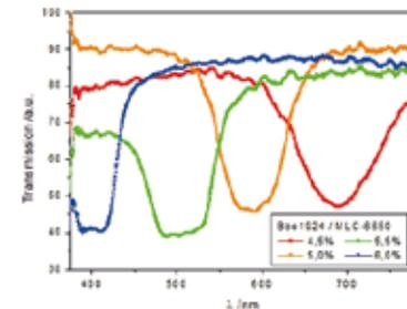
3 Adjustment of reflection wavelength by the concentration of the chiral dopant
