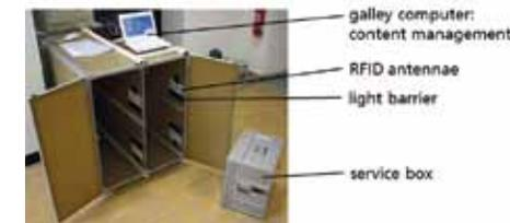
4 Mock-up of a novel galley compartment with galley control unit
