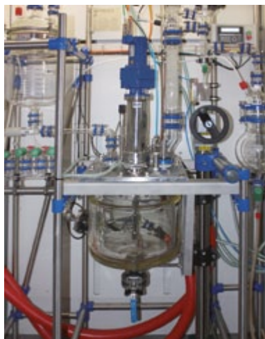
1: 20 kg condensation plant
