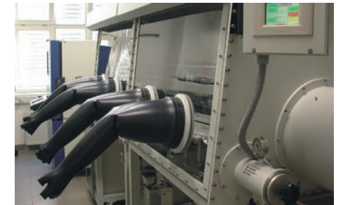
6 Glovebox for the encapsulation of test cells
