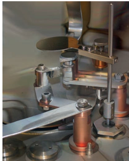
1 Vaporizer for the application of calcium layers
