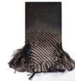
6: CF-reinforced laminate with partly removed thermoset
