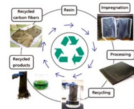
7: Recycling loop of CF-reinforced laminates
