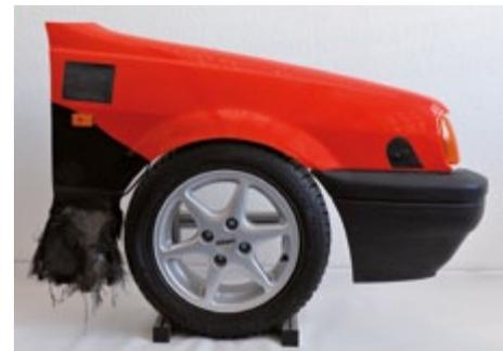
1: Recycling and repair of a CFK-fender with thermoset matrix (© Torsten George)
