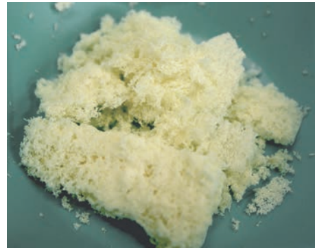
6 Partly decomposed foam after immersion in chemical substance for 60 min
