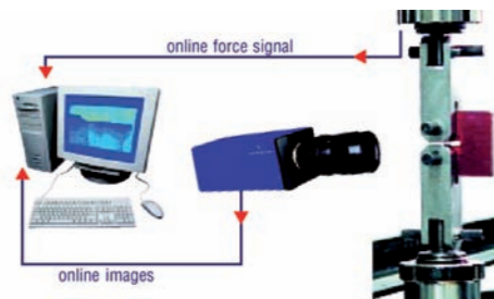
1+2 Optical Crack Tracing with digital video camera
