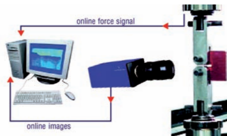
1+2 Optical Crack Tracing with digital video camera
