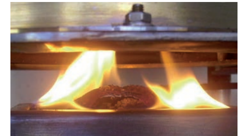
6 Char layer covered sample surface
