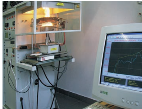
8 Fire test in the cone calorimeter, with the combustion process being presented simultaneously
