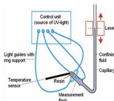
Fig. 4: Setup of a volume dilatometer for light-curing resins.
