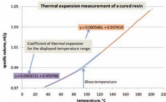
**Fig. 8:** Volume dilatometric measurement of the thermal expansion.
