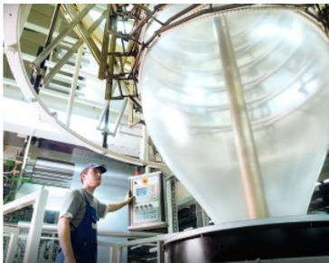
Together with 18 partners from industry and research, Fraunhofer IAP is developing new types of polybutylene succinate in the RUBIO project. The bioplastic is being optimized for new application areas. The first marketable product was created in collaboration with Polifilm Extrusion GmbH.
